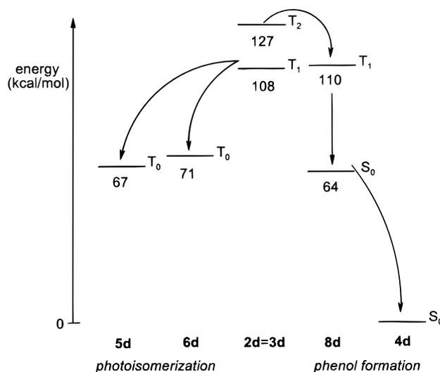
**Figure 2.** Computed energy diagram of intermediates and products of the model system **2d** = **3d** (arrows correspond to most likely processes; S<sub>0</sub> of **4d** was set to 0 kcal/mol).
