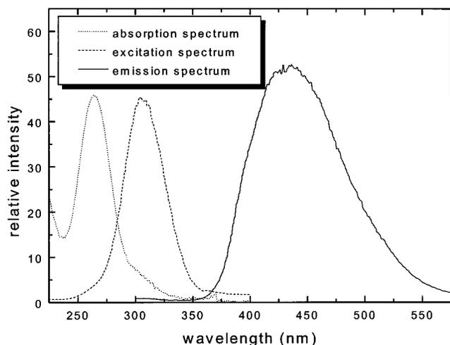
**Figure 1.** Spectral overlay for compound **2a** (absorption spectrum (reduced for graphic reasons) in methanol at 298 K with  $\lambda_{\max} = 264$  nm, phosphorescence excitation spectrum at  $\lambda_{\text{em}} = 430$  nm in ethanol at 77 K with  $\lambda_{\max} = 305$  nm, and phosphorescence emission spectrum at  $\lambda_{\text{exc}} = 300$  nm in ethanol at 77 K with  $\lambda_{\max} \approx 433$  nm).
