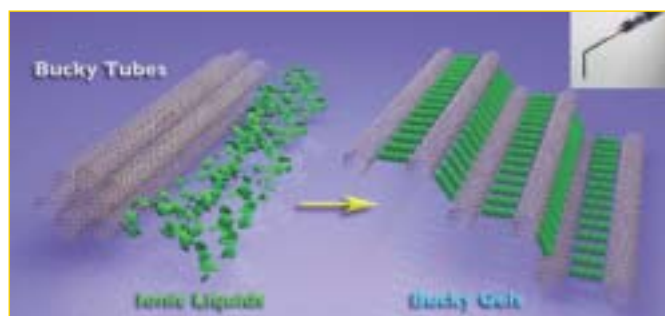
'Bucky gels' SWNTs dispersed in an ionic liquids (inset shows extrusion through syringe).
