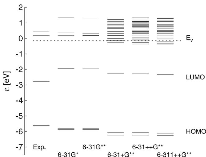
FIGURE 7 Energetic positions of MOs of *trans*-TBA for different basis sets at the B3LYP level of theory
