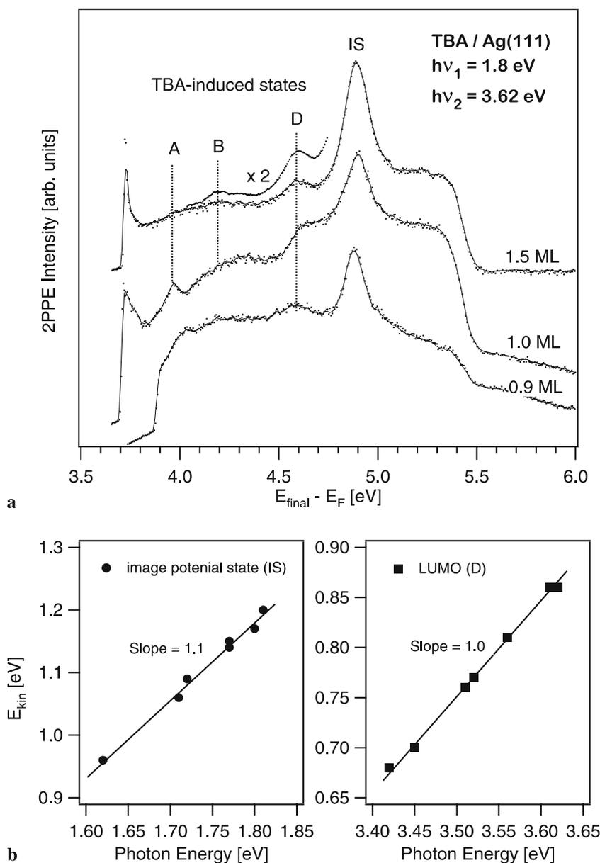
**FIGURE 5** (a) Two-color 2PPE of Ag(111) at different TBA coverages measured with 1.8 and 3.62 eV photons. (b) Photon energy dependence of the peaks D and IS from 1.5 ML, in the 2PPE spectra of TBA/Ag(111). The symbols are experimental data, and the *solid lines* are fitting curves. The kinetic energies of both peaks D and IS vary with  $1\Delta h\nu$ , indicating that they originate from unoccupied intermediate states in the 2PPE process
