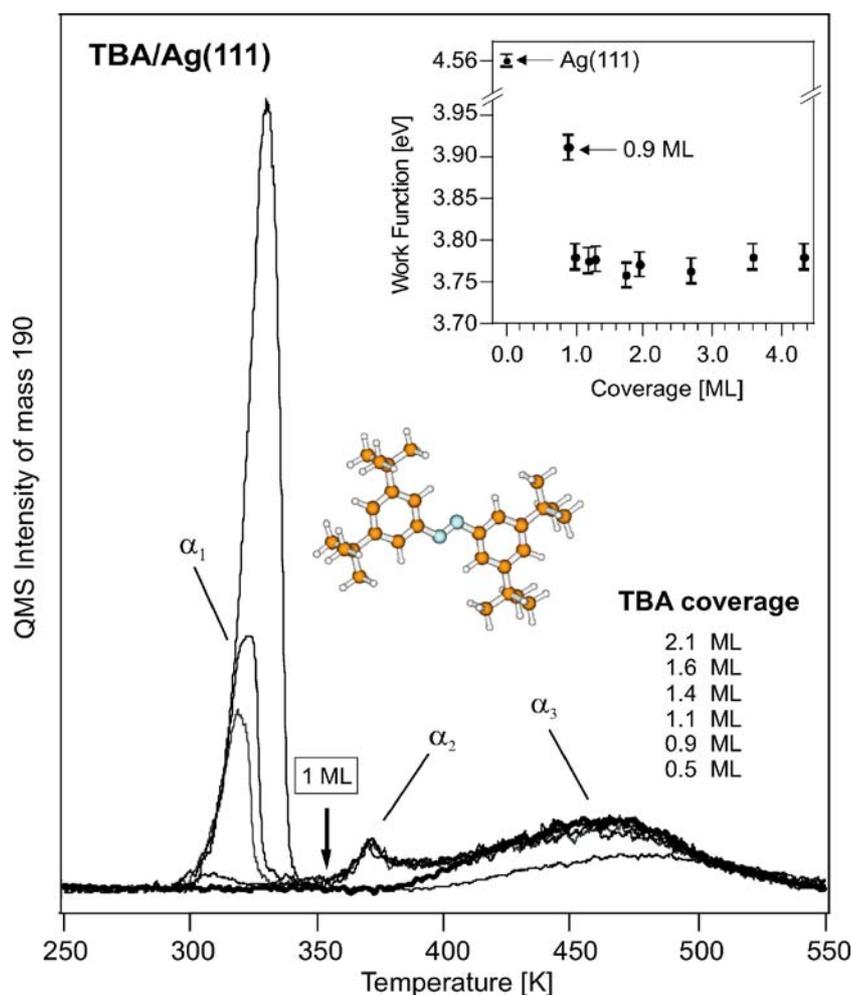
**FIGURE 1** Thermal desorption spectra of TBA on Ag(111) at different coverages. The *thicker solid line* represents a coverage of 0.9 ML. The *inset* shows the work function of TBA/Ag(111) as a function of coverage, determined by the low energy cutoff in the 2PPE spectroscopy
