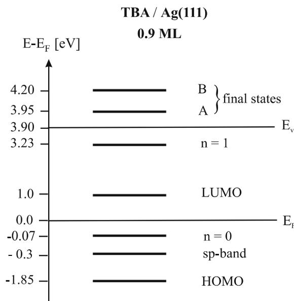
**FIGURE 6** The energies of the observed photoemission spectral features in TBA adsorbed on Ag(111). All features are referenced to the Fermi level of Ag(111)
