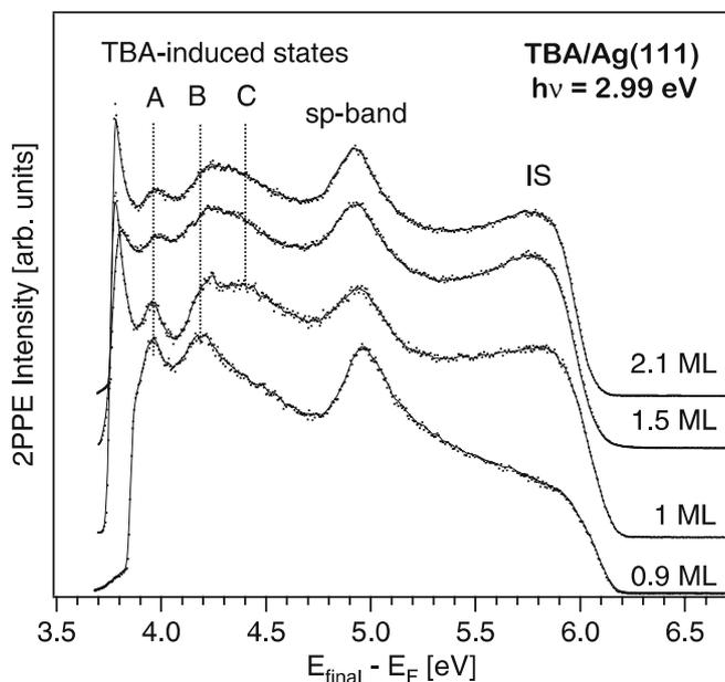
**FIGURE 3** One-color 2PPE spectra taken at a photon energy of 2.99 eV for the TBA-covered Ag(111) surface at various coverages. The spectra are displayed as a function of final state energy above the Fermi level,  $E_{\text{final}} - E_{\text{F}} = E_{\text{kin}} + \Phi$ . Major features are labeled as A, B, C, and IS. For their assignment see text
