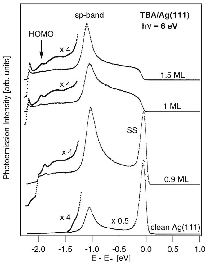
**FIGURE 2** Ultraviolet-photoemission spectra received at a photon energy of 6 eV from the clean and TBA-covered Ag(111)
